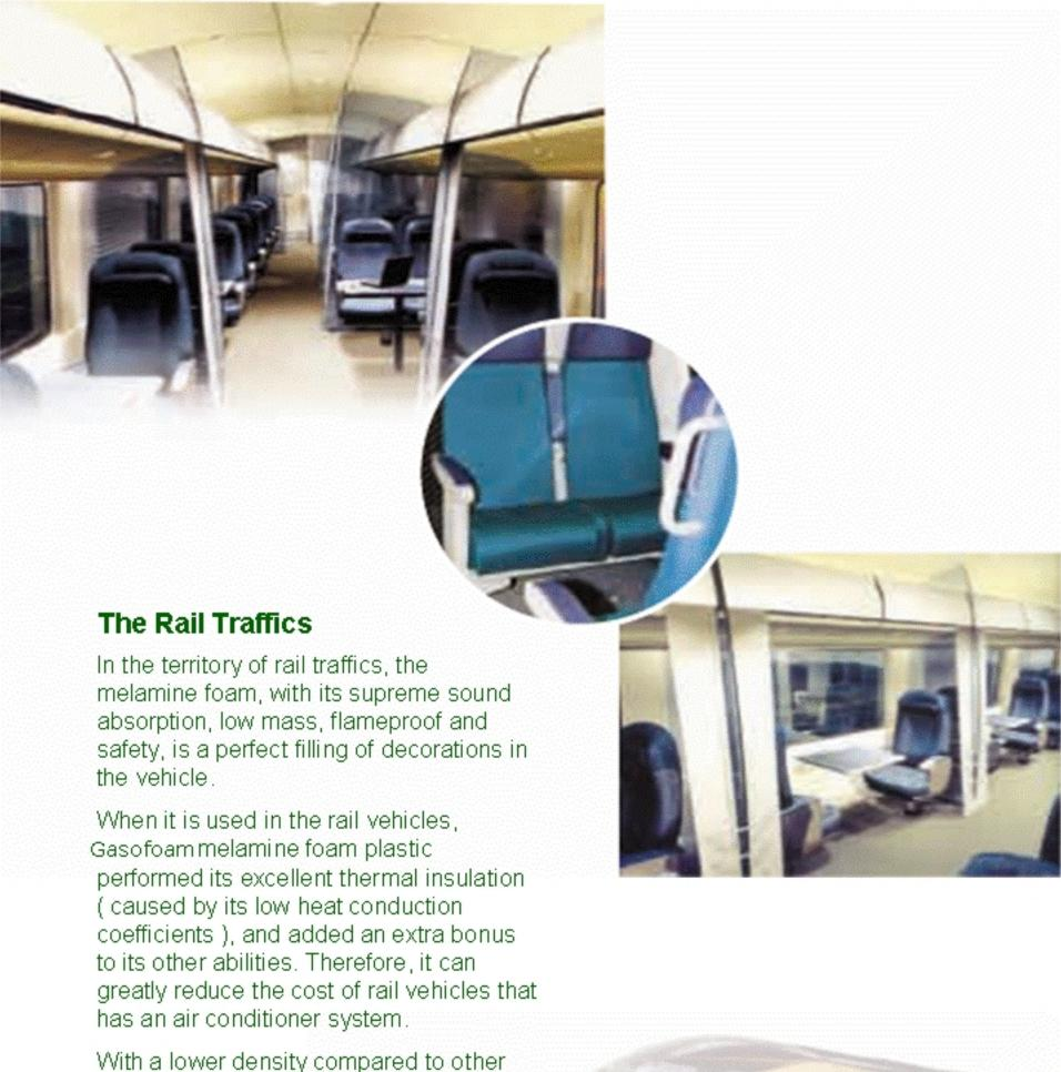
With a lower density compared to other soundproof materials, the appliance of Gasofoam melamine saved energy for the vehicle itself. In addition, the decrease of weight of the ceilings and walls of the rail vehicle increased the safety when the vehicle turns, because of a lower centre of gravity. This is particularly significant for narrow-gage railroads.
